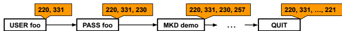
Fig. 3. An annotated FTP message sequence processed for mutational fuzzing (from the sniffer trace in Listing 1).
