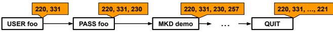
Fig. 3. An annotated FTP message sequence processed for mutational fuzzing (from the sniffer trace in Listing 1)
