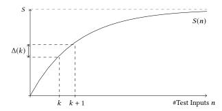
Figure 1: The expected number S(n) of program behaviors that a test generator discovers as the number of generated test inputs n increases. The rate  $\Delta(n) = S(n+1) - S(n)$  at which behaviors are discovered decreases over time. Function  $\Delta(n)$  gives the *current* discovery rate when the n-th test is generated. In the limit, the expected number of behaviors discovered approaches the asymptote S.
