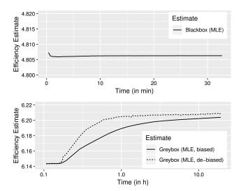
Figure 3: Entropy estimates of a blackbox fuzzer's entropy (top) and a greybox fuzzer's entropy (bottom) over time. For each species  $\mathcal{D}_i$ , we count the number of generated inputs  $Y_i$  belonging to  $\mathcal{D}_i$  and in regular intervals compute  $\hat{H}_{\text{MLE}}$  per Eqn. (15). For the de-biased estimator (bottom), we reset the incidence frequencies  $Y_i = 0$  whenever a new seed is added.
