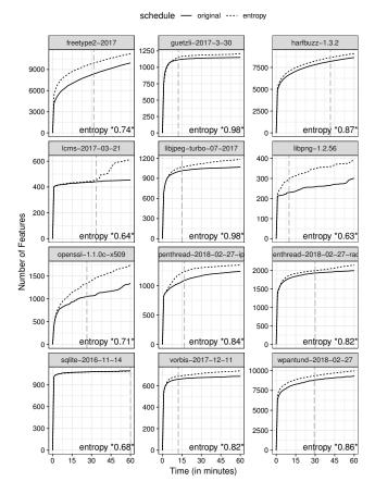
Figure 5: Mean coverage in a 60 minute fuzzing campaign (12 subjects  $\times$  2 schedules  $\times$  40 runs  $\times$  1 hour  $\approx$  40 CPU days). The dashed, vertical lines show when Entropic achieves the same coverage as LibFuzzer in 1 hour. The values at the bottom right give the Vargha-Delaney effect size  $\hat{A}_{12}$ .
