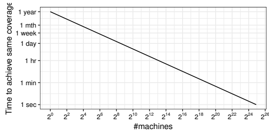
Figure 11: Second law. We observe an exponential decrease in the time spent to discover the same number of species with an exponential increase in available machines (i.e., in the number of test cases that can be generated per minute).
